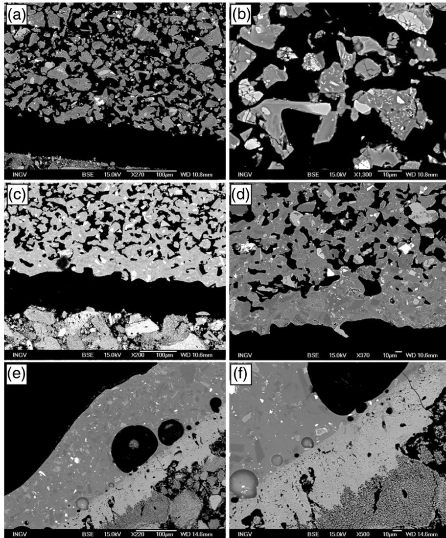
**Figure 3** SEM images of impregnated thin section showing the different degrees of sintering from quasi-initial conditions after 60 minutes at 950°C (a overview, b detail), through considerable neck formation after 60 minutes at 1000°C (c overview, d detail) to complete textural densification after 60 minutes at 1050°C (e overview, f detail).
