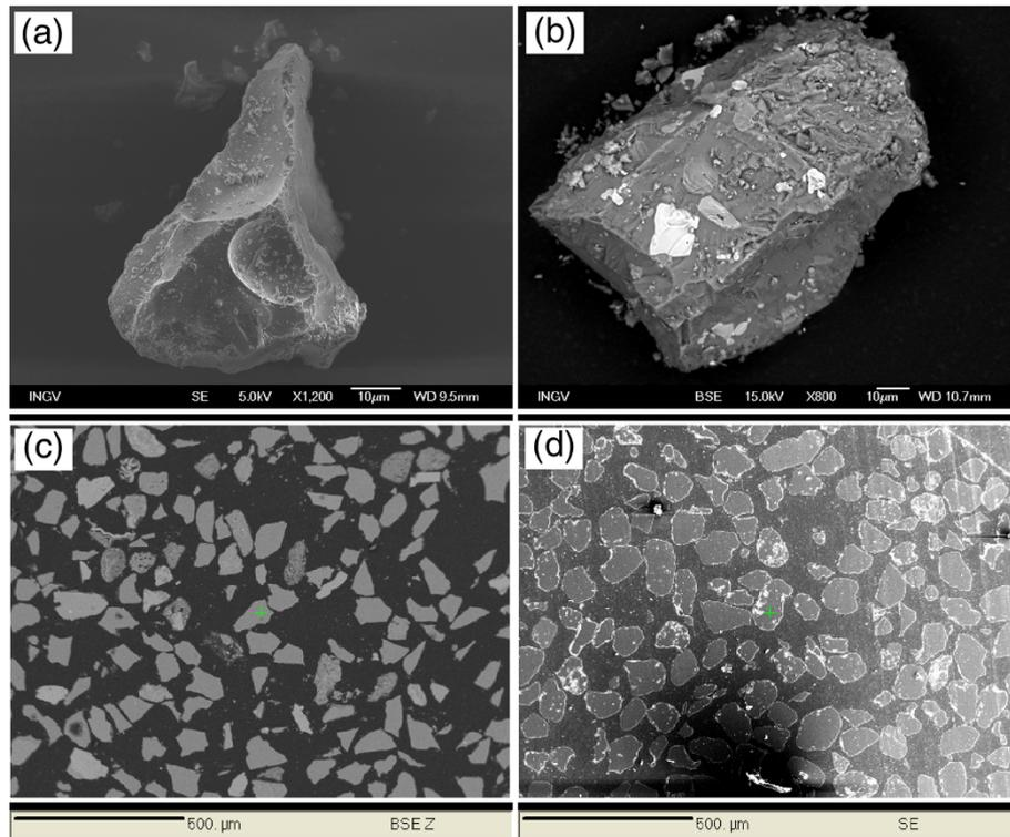
**Figure 1** SEM images of single and embedded grains. **a)** and **b)** showing different EYJA grains showing the porous nature **(a)** and the microlite content **(b)**; **c)** shows the angular shape of ATD grains; **d)** shows the rounded shape of MIL grains.
