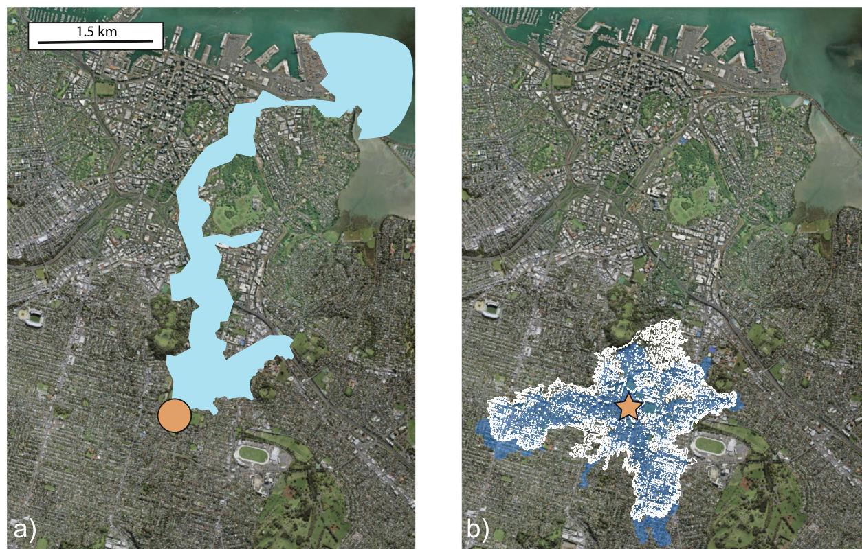
Fig. 4 Comparison of the Mt Eden lava flows created a) for Hayes et al. (2018) where the lava flow effuses from the bottom of the cone (a large area represented by the brown circle) and b) using MOLASSES where the lava flow effuses from a point source vent (orange star)
