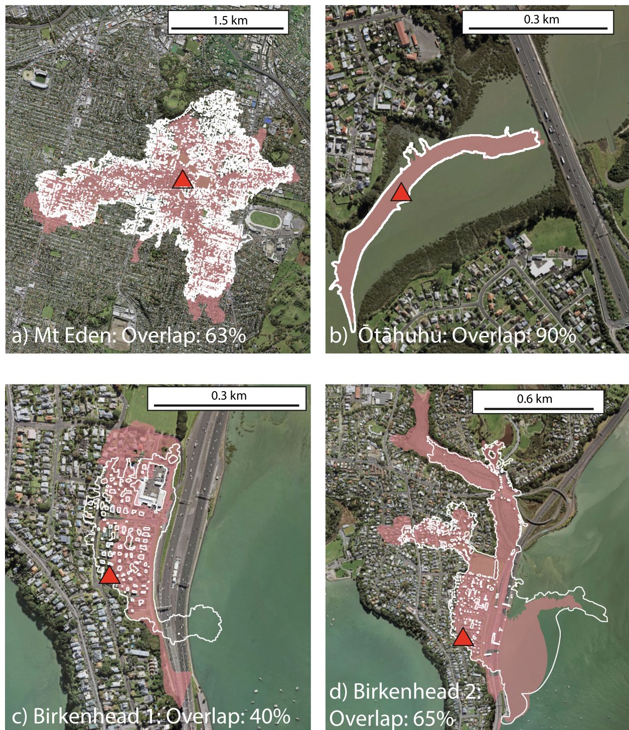
Fig. 2 Results of lava flow modelling using MOLASSES on a DEM (results shown in pink) and a DSM (results outlined in white) with scenario vent indicated with a red triangle for a ) the Mt Eden scenario, b ) the Ōtāhuhu scenario, c ) the first lava flow in the Birkenhead scenario and d ) the second lava flow in the Birkenhead scenario. Note different scales in each figure. Percentages refer to the modified Jaccard coefficient calculated for each scenario
