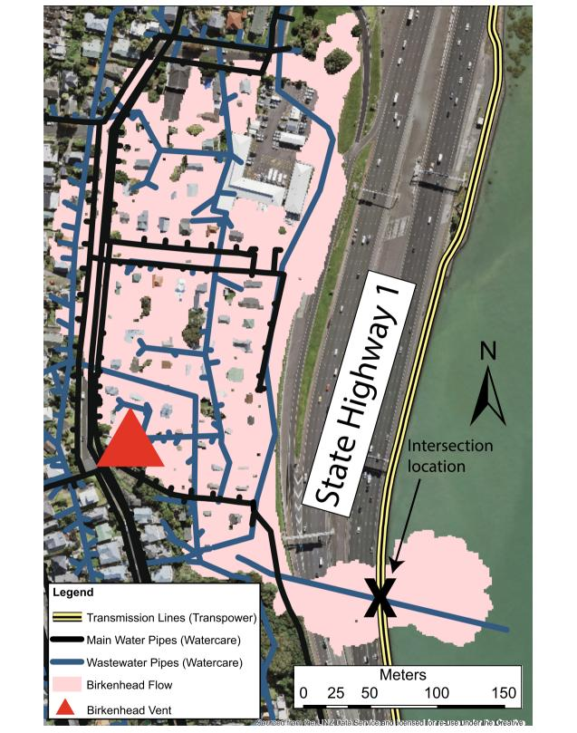
Fig. 3 Map of areal footprint (modelled with MOLASSES) and buried infrastructure networks in the Birkenhead suburb on Auckland's North Shore. Infrastructure data publicly available from Transpower New Zealand (2019) and Watercare Services Ltd. (2019)
