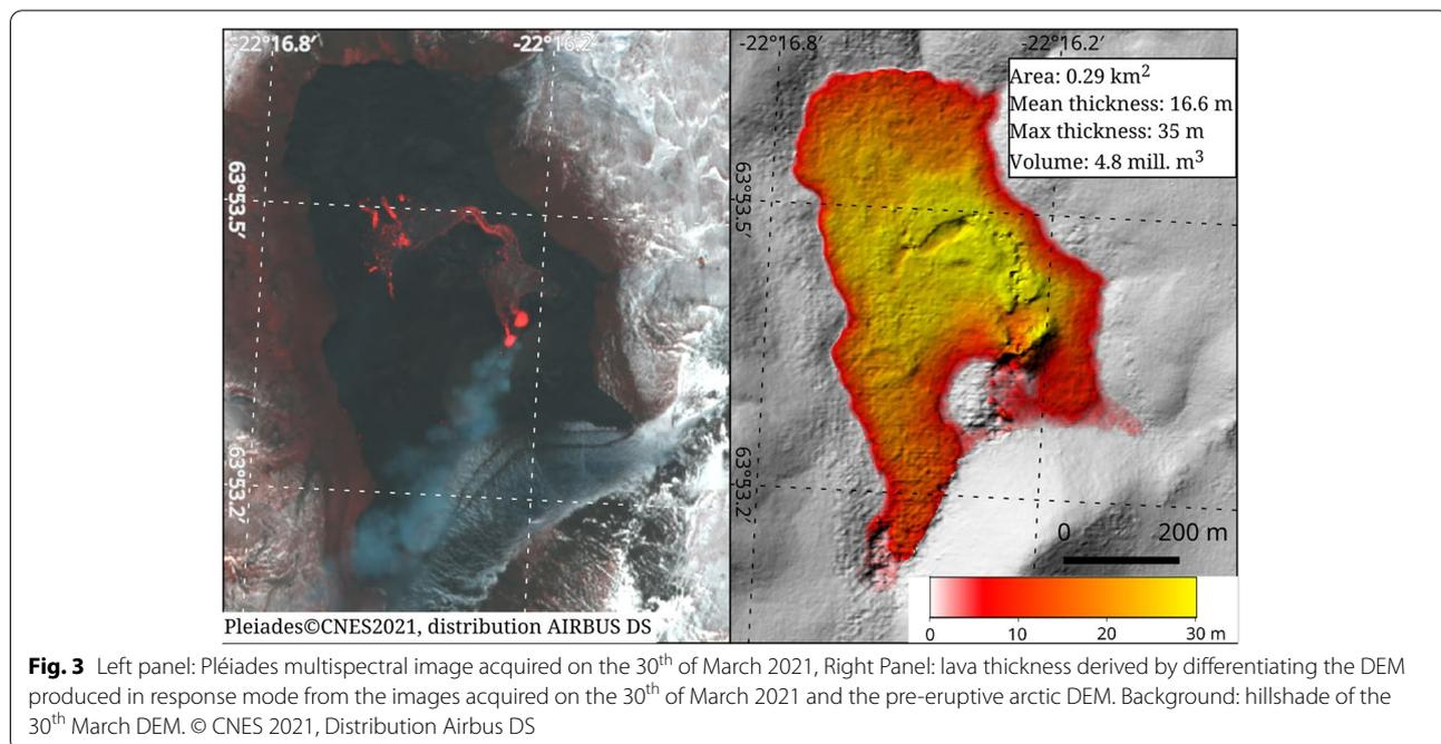
**Fig. 3** Left panel: Pléiades multispectral image acquired on the 30<sup>th</sup> of March 2021, Right Panel: lava thickness derived by differentiating the DEM produced in response mode from the images acquired on the 30<sup>th</sup> of March 2021 and the pre-eruptive arctic DEM. Background: hillshade of the 30<sup>th</sup> March DEM. © CNES 2021, Distribution Airbus DS
