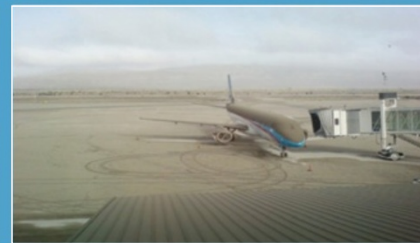
5-10 mm of ash fall at San Carlos de Bariloche International Airport in Bariloche, Argentina, following the June 2011 eruption of Peñufoe Cordón-Caulle volcano in Chile. The airport closed for 31 days due to the on-going ash falls, remobilisation of ash and cleanup.
