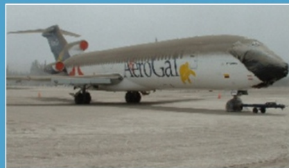
3-5 mm of ash fall at Mariscal Sucre International Airport in Quito, Ecuador, following the 3 November 2002 eruption of Reventador volcano. The airport closed for 8 days due to the ash deposition on aircraft and runways.
