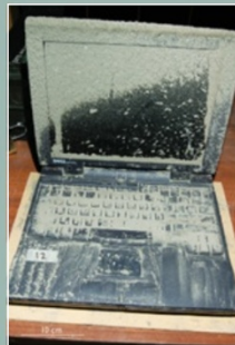
Reducing the exposure of computer equipment to ashfall is the most effective mitigation action. Experiments suggest that laptops may shut down due to overheating when covered in ash, but relatively little enters the internal compartment. After cleaning, the laptop shown in this experiment restarted successfully.
