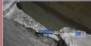
Accelerated abrasion damage to wicket gates from Agyan HEP, Ecuador. Normal design life of turbines at this plant is 6-7 years, but this has been reduced to 5 years due to ashfalls from nearby Tungurahua volcano contaminating reservoir water.
