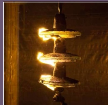
3 mm of ash fall cover on a glass insulator string inducing a flashover. Note how the current is tracking through the volcanic ash covered insulator surface
