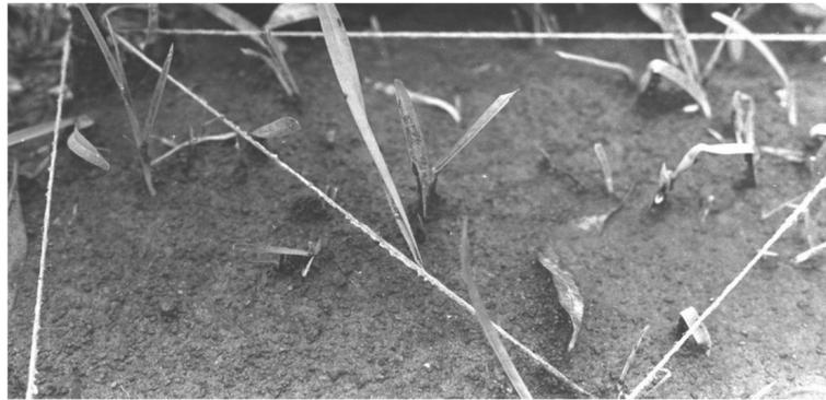
**Fig. 5** Part of Plot 2 16 days after the start of the experiment. Compaction by raindrop impact is evident as the taut strings, initially flush with the tephra surface, stand proud. Numerous grass shoots have penetrated the tephra surface. The initial thickness of 50 mm has been reduced to 25–30 mm in just 16 days
